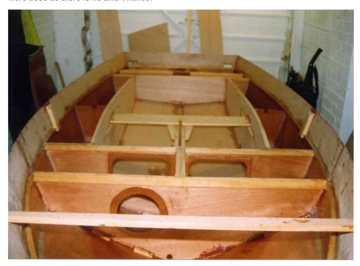
The final step is fixing the decks to the hull. By this stage all the internal structure is complete and the tanks coated in epoxy. The fitting of the decks suddenly makes the kit look like a boat.
