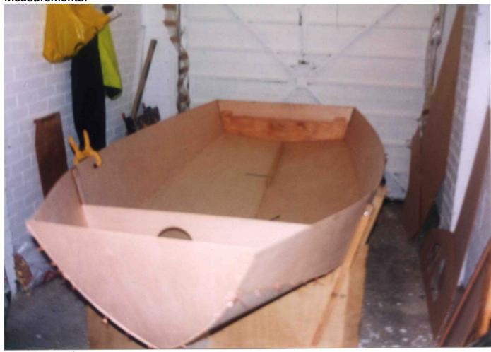
The 1st pieces to be fixed are the bulk heads. These form the shape at the front of the boat and it is preferable to glue these prior to taping the seams. Note that a string line has been set up to ensure the boat remained straight throughout the building process. The centreboard was also fixed at this stage, Like most fast mirrors we fixed this as far back as possible under the rules.
