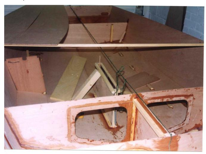
This photo shows the rear deck support glued into place and the seams taped prior to fixing the rear deck. The tank is also coated in epoxy.
