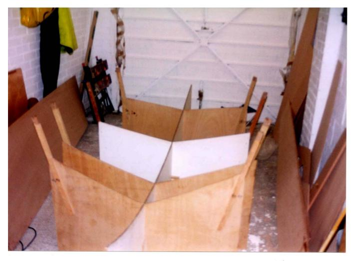
The Main Panels were fixed to the Jig, requiring minor reshaping of the supplied panels to make best use of the tolerances within the Mirror class rules. All the top boats now follow a similar principle of flat aft sections and maximum curvature, and hence buoyancy, towards the front. It is practical to make the jig to match an existing boat's measurements.
