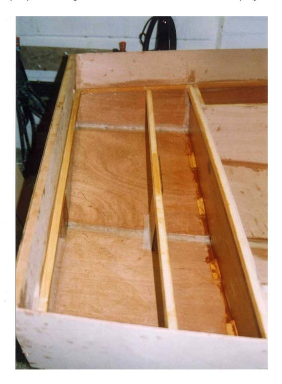
This photo shows the forward tank and bulkhead prior to fixing the fore deck. The battens that support the deck are in place and all the taped seamed.
