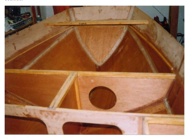
The side tanks just prior to deck Fixing. Note that the bulkhead needs to be fixed directly in line with the thwart.
