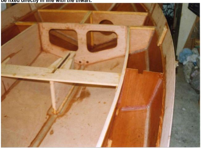
This Pictures shows the boat prior to fitting the decks. By this stage all the bulk heads and thwart had been glued in and all the seams taped. The temporary strut at the front held the bow in shape prior to fixing the decks. You will see that all the tanks have been coated in West. 3 coats were used as there is no 2nd Chance!
